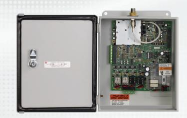
The Federal Controller, model FC, is a remote control activation point for control of equipment with timer and relay outputs. Optional radio/receiver decoder is available. This versatile model is ideal for virtually all siren control applications and any other process that can be controlled via relay contacts.
